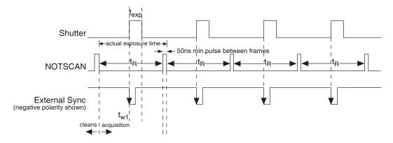
Figure 16. Frame Transfer where  $t_{w1} + t_{exp} + t_c < t_R$
